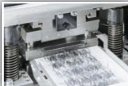
In the second tool station, the concrete steel fibres are cut to the correct length. The blades are made of carbide, thus ensuring a long service life. A conveyor belt carries away the concrete steel fibres from the machine area.
