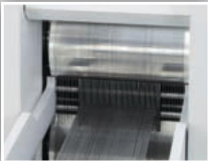
A robustly designed mill draws the wires directly from the coils through a straightening mechanism. Depending on the wire quality, a minimum rolling depth of 0,1 to 0,2 mm is required.
