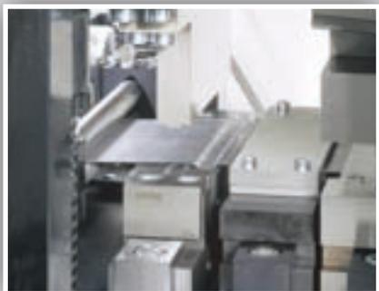
In the first tool station, the wires are bent. This bending gives the concrete steel fibres the typical Z-hooks that can then be anchored in the concrete.
